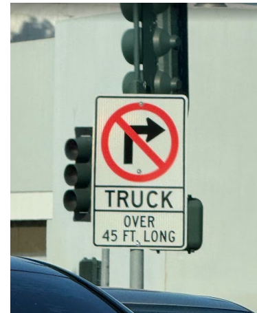
Sample signage for truck size limits and prohibited routes
